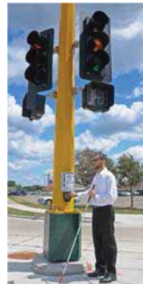
Figure 23-22: An Accessible Pedestrian Signal
