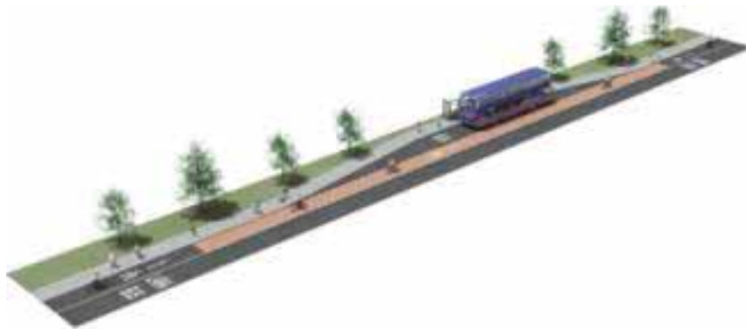
Figure 23.13:– Typical layout of a bus bay (For illustrative purpose)
